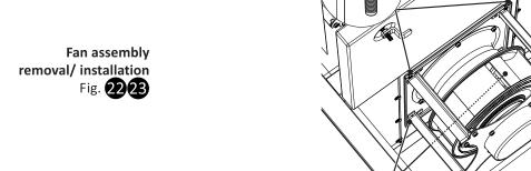
To replace the fan assembly, locate the mounting plate over the fixings retained in the unit bulkhead. Secure the loose fixings through the mounting plate and tighten all the mounting fixings. Reconnect the supply plugs as in Fig. 3; if more than one plug is used, ensure the correct plugs are reconnected as marked. Ensure that the fans are free running by following the fan alignment instructions in Fig. 24 on page 13, adjust as required.
