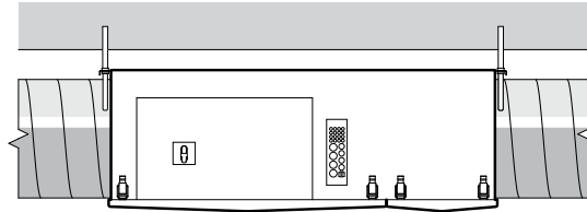
3 Plantroom ceiling mounted (fan, filter & control panel option shown)
