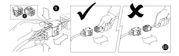
On reconnection, the assembly features a locating lug to ensure correct orientation. Once rejoined, lock the connection together again using the corresponding system as shown. Note the plugs are handed and forcing an incorrect connection may result in damage to the plug.
