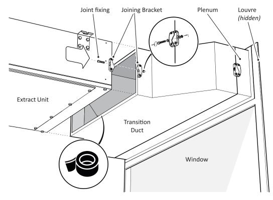
Fix the bracket parts to both sides of unit and transition as shown using the M6 fixings provided. Tape the joint using self-adhesive rubber tape prior to assembly to prevent air leakage.
