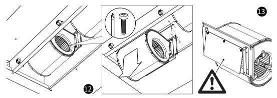
Extract Fan assembly removal/installation
