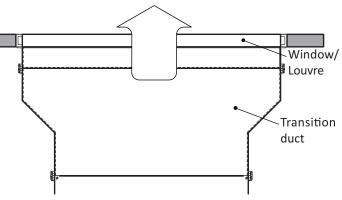
Duct transitions and plenum boxes allow for resizing and/or realignment as required and should be sized to match both unit and louvre connections. A pair of joining brackets per section (one each side) are provided to assist with the duct connection.
