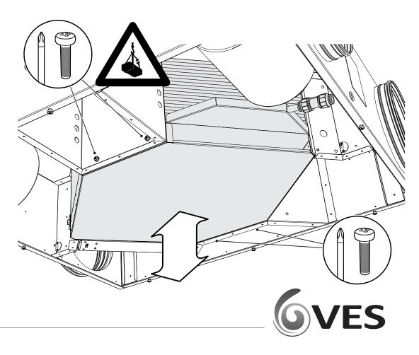
Bypass/Heat exchanger removal
