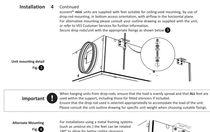
180° to allow for better ceiling clearance. Carefully remove/retain the fixings and reposition the feet as required. Ensure all fixings are correctly reinstated and tighten to 8Nm.
