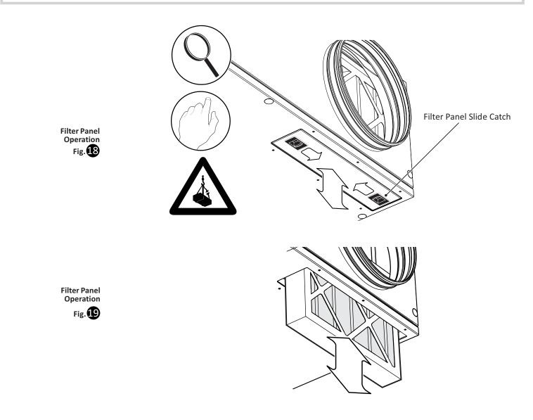
To replace, dispose of the old filters responsibly, note the airflow direction arrow on the new filter. Slide the clean filter into the unit and replace the filter doors.
