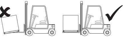
Handle with care. Failure to fully support the unit during lifting may result in damage to the unit.
