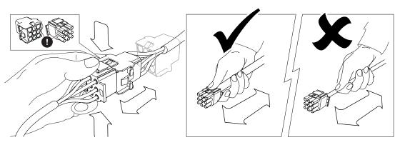
On reconnection, the assembly features a locating lug to ensure correct orientation. Once rejoined, lock the connection together again using the system as shown. Note the plugs are handed and forcing an incorrect connection may result in damage to the plug.
