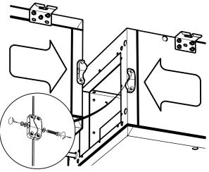
Joining brackets are **NOT** structural and are included as part of the unit sealing only. When moving assembled units ensure that **ALL** sections are fully supported.
